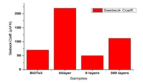
Fig. 3: variation of seebeck coefficient with thickness.
