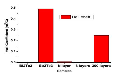
Fig.1.3: Variation in Hall Coefficient with Thickness
