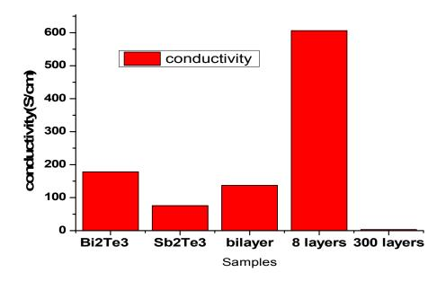
Fig. 1.4: Variation in Conductivity with Thickness
