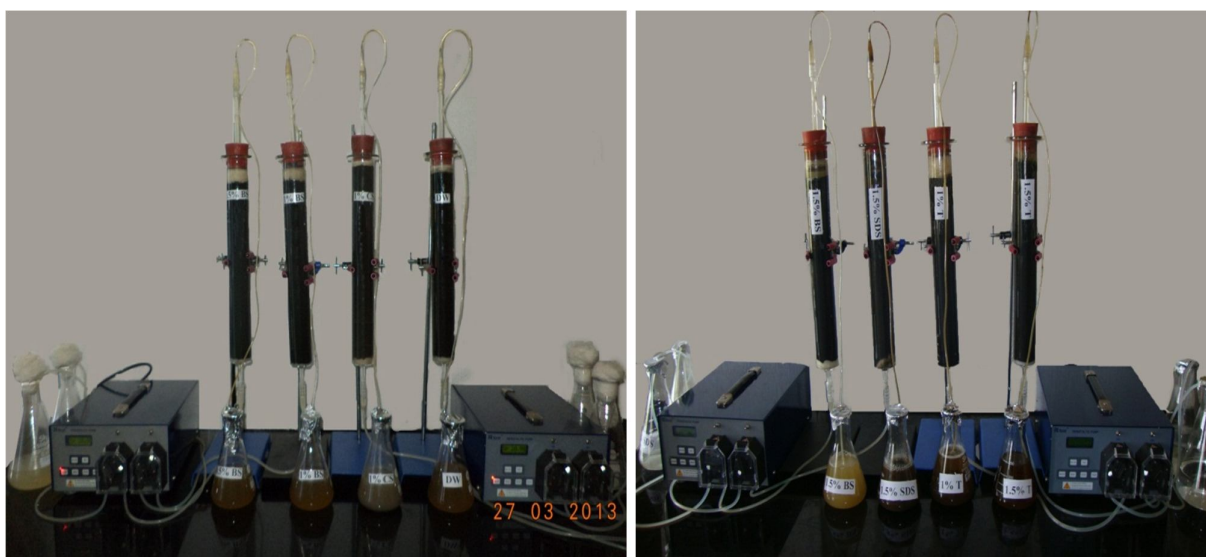
Fig. 1: Bioremediation of crude oil contaminated soil by soil column process
